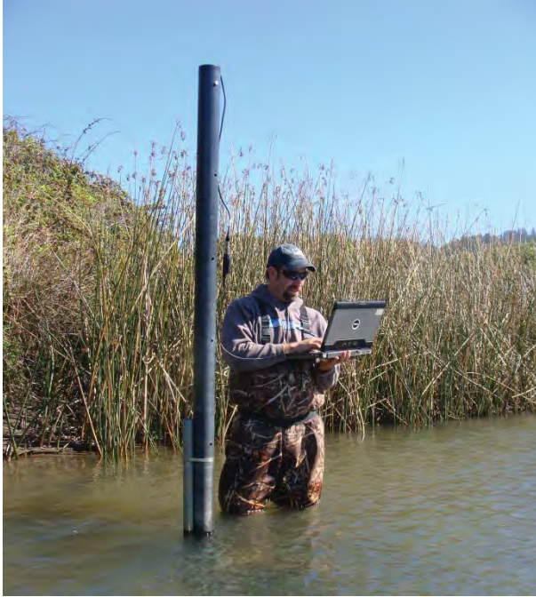
Picture of water level recorder in a stilling well taken at low tide.
